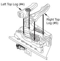
Figure 28 - Installing Top Logs
